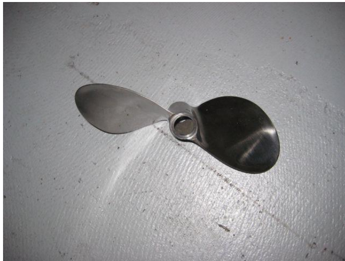
This is a Hill Marine Prop that works very well for Solar Cup (Stainless steel, variable pitch, racing prop)
