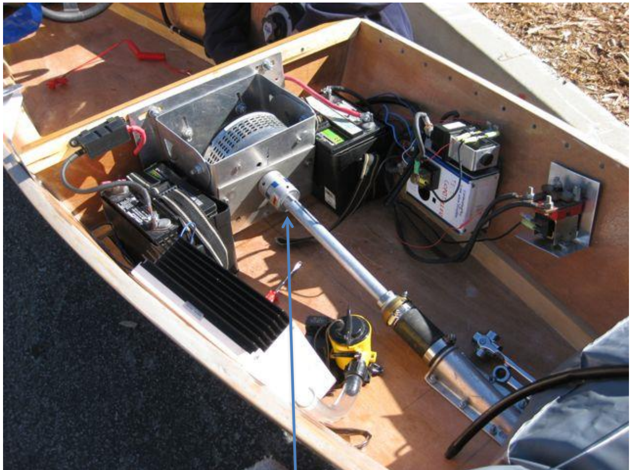
Motor mount and Lovejoy coupler for direct drive (no transmission)
