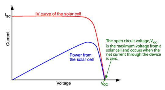
The graph above shows the output of the solar panel is not linear across the range. As the resistance changes, the voltage holds almost the same until the voltage reaches a critical level. The current then starts to decrease at a high rate, until it is 0 at the Open Circuit
