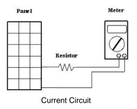
a. Hook up the circuit as shown above using the breadboard and one of the resistors.
