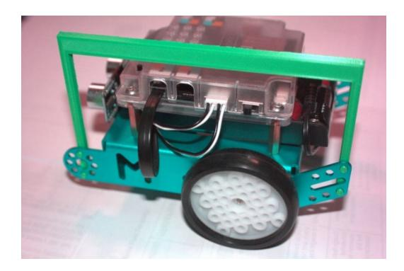
6. Here is a picture of a platform which fits nicely along the top of the robot and attaches to arms on the front and the back.
