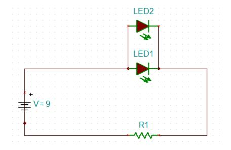
Use the formula above to find the value of R, and then build the circuit shown above. Be sure to use the same color LED's, don't mix colors. Because of the increased current in the circuit the resistor R1 may overheat if you leave it connected too long, or if the value of R1 is not correct. If the resistor overheats (it may smell funny too) disconnect the battery and let it cool down.
