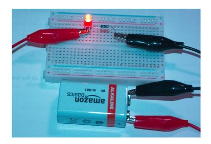
Note that the LED is polarized, that is, it has a plus and minus lead as shown in the picture below. The plus side of the LED must be connected to the plus (+) side of the battery. If you think your circuit is correct but the LED won't light up, try reversing the LED in the breadboard.
