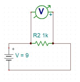
6. The meter in the picture below is measuring the voltage drop across the resistor. You can see that the green and red alligator clips are hooked up to the meter leads are across the resistor.
